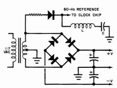
quired rejection. However, if the signal is very strong, it could cause the counting circuitry to act up. If this is the case, install the series-tuned LC trap shown in the figure at the 60-Hz reference tap-off. U,se a  $0.02-\mu F$ , 75-V ceramic capacitor (Lafayette 33 F 69063) for C and a 1-10-mH width coil (Miller 6322, Lafayette 34 F 88525) for L. Adjust L for normal clock counting.
